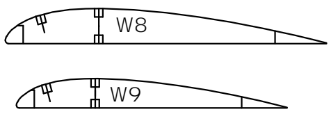
All wing ribs from 1.6mm sheet
